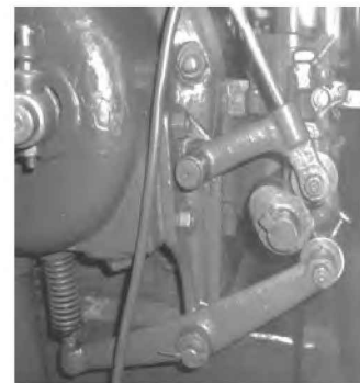
A cam with two oscillating followers. This cam operates the inlet as well as the exhaust valves of the engine
