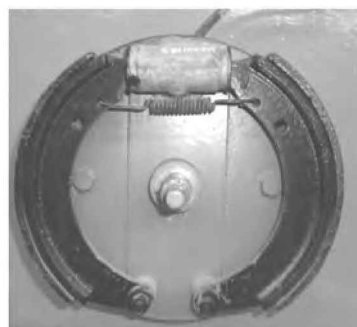
Internal expanding shoe brake mechanism (without brake drum).
