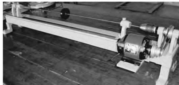
Lab set up to find the whirling speed of shafts
