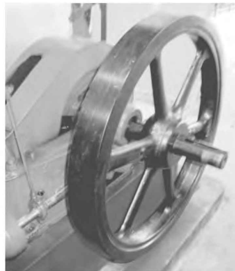
Flywheel of a diesel engine
